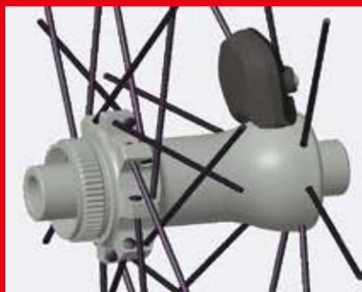
Do not mount sensor on drive side.
