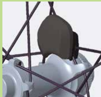
Position sensor as close to the hub axis as possible.
