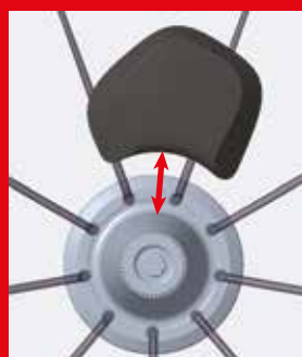
Do not mount sensor far from hub axis.
